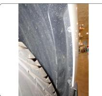
2. Disconnect fascia clips from under taillights to remove fascia. Gently pull fascia away from vehicle, making sure to carefully disconnect electrical connectors during removal. Set aside parts for reassembly.
