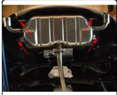
2) Remove the tape if present from the forward most attachment point and fishwire the (2) supplied carriage bolts and (2) sp-6 spacers on both sides. Reverse pull the remaining (2) bolts and (2) spacers on both sides into the rearward attachment holes. Leave the wires on temporarily while raising hitch (refer to diagrams to the left for fishwiring techniques).
