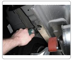
**FISHWIRE TECHNIQUE** INSERT COILED END OF FISHWIRE TOOL THROUGH HITCH MOUNTING HOLE IN VEHICLE FRAME RAIL AND OUT THE ACCESS HOLE. PASS COILED END OF FISHWIRE THROUGH SPACER AND THREAD BOLT INTO COIL. KINK WIRE TO KEEP SPACER SEPERATE FROM BOLT AS SHOWN. PULL FISHWIRE, SPACER, AND BOLT THROUGH FRAME AND OUT MOUNTING HOLE. USE FISHWIRE TO GUIDE HITCH DURING MOUNTING AND PREVENT LOSS OF BOLT SPACER INSIDE FRAME RAIL. \*\*NOTE: SOME VEHICLES MAY FISHWIRE THROUGH END OF FRAME
