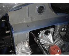
4. Raise hitch into position and loosely secure the rear most holes with 7/16"-14 flange nuts. Place the hitch side plates against the frame rails, followed buy 11431-SP, and then the exhaust brackets. Secure with supplied M8-1.25 hex bolts and 3/8" conical toothed washers.
