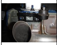
2. Temporarily remove the heat shield using a needle nose pliers to remove the (6) retention nuts. Trim heat shield following contours as shown removing a 3" x 3" square using Trim Diagram below as reference.
