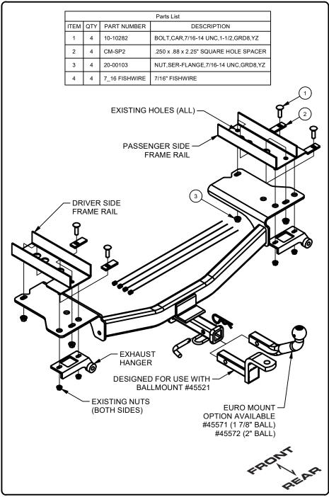
1. Lower exhaust by using a 13mm socket to remove (2) nuts from each exhaust hanger. There is a plastic clip on the exhaust hanger that needs to be pushed out of the way to allow the exhaust to be lowered.
