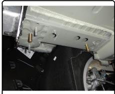
4. Raise hitch into position over exhaust and secure with 7/16" flange nuts. Torque 7/16" bolts to 59 ft-lbs. Reinstall exhaust using nuts removed in Step 1.
