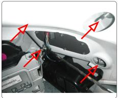
10. Disconnect the wiring harness from each taillight.
