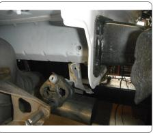
15. Remove (2) outer bumper beam hex flange nuts using a 16mm socket. Repeat on other side.
