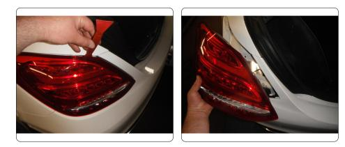
12. Carefully remove bumper cover. Start by pulling the outer edges near wheel wells and proceed rearward until cover is removed. If present, unplug and remove wire harness from the inside of bumper cover.
