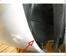
3. Remove (1) hex head screw upper area of each wheel well using an 8mm socket. NOTE: They are located under wheel the well liners.
