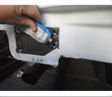
Raise hitch and bumper beam into position and attach to outer (4) bumper beam studs using the existing M10 flange nuts.
