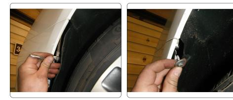
4. Open trunk and remove (1) plastic hook per side. Use a flathead screwdriver to remove center rectangular head pin and then remove hook.
