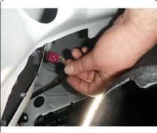
11. Carefully pull taillight rearward and remove, repeat on other side. Use a trim panel tool to ease the process.
