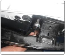
23. Use tape measure, marker and cut wheel to remove a 1.63" wide x 1.25" deep rectangle from center bottom portion of fascia panel.
