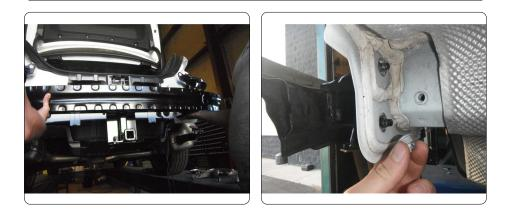
20. Insert (4) supplied M10 hex bolts with (4) M10 washers through bumper beam, hitch and vehicle.
