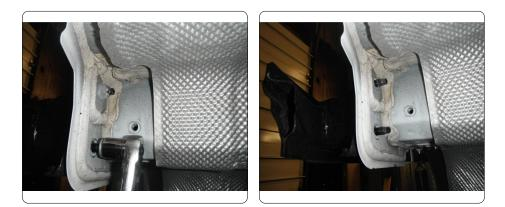
Remove (4) inner bumper beam hex flange nuts using a 16mm socket. These are located inside the trunk under the floor liner. Remove bumper beam.
