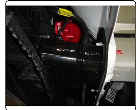
2. Fishwire 7/16" carriage bolts and 11529-SP spacers into lower holes in the outside of the frame rails.
