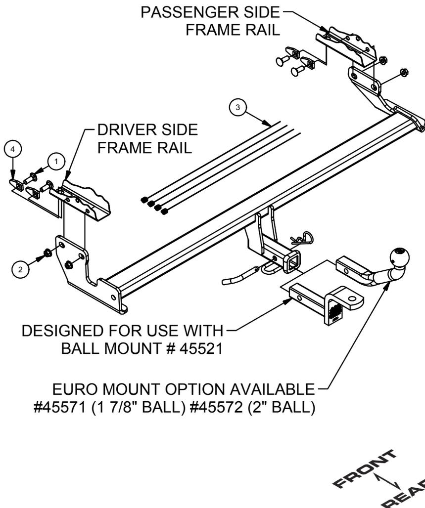
1. Relocate electrical harness from under the driver side of the bumper beam to above the bumper beam. Remove underbody panel from passenger side frame rail. Save for reinstallation in Step 4.
