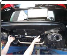
6. Torque all 7/16" hardware to 70 ft-lbs and 3/8" hardware to 45 ft-lbs. (If present) Trim underbody panel then slide hitch bracket through trimmed section. Raise underbody panel into position and reinstall fasteners.
