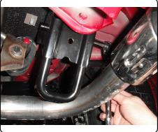
2. Insert 1/2-13 x 4 1/2" carriage bolts and CM-12048-SP spacers through the existing holes in the side of the frame rails. After bolts are inserted push them back so the end is flush with the inside of the frame rails. Temporary lowering of the charcoal canister on the driver side will ease installation.
