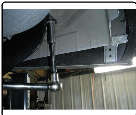
5. Replace rubber plugs in trunk pan and tuck carpet back into original position.
