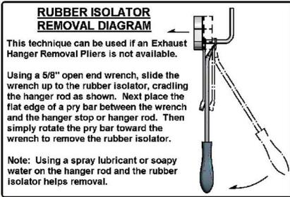
1.) Lower exhaust by removing rubber isolators (3 each side) as shown.
