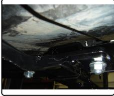
9. Raise nut plate in front of vehicle crossmember. Loosely secure nut plate to mounting strap with 1/2-13 x 2 1/2" hex bolts and 1/2" conical toothed washers.
