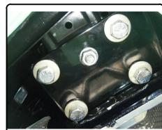
8. Insert 7/16-14 x 1" carriage bolts through top of square holes behind receiver tube of hitch. Raise mounting strap between vehicle crossmember. Loosely secure mounting strap to hitch with 7/16" flange nuts.
