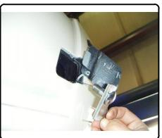
6. Place supplied nut plates over bumper beam. Raise hitch into position over exhaust and loosely secure hitch into place with 7/16" flange nuts. **Note:** Be sure to slide hitch as far forward as possible but not so it rests on the weld seam on the vehicle bumper beams.
