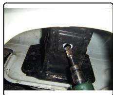
4. Locate channel behind driver side bumper fascia leading to access hole in driver side bumper beam. Fishwire 7/16-14 x 1 1/4" carriage bolt and SP2 spacer through access hole and out enlarged hole in driver side bumper beam.
