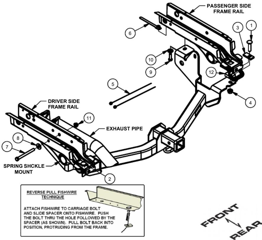
1. Remove the rearwardmost rubber plugs in the frame rails and foil (if present) covering the mounting holes. Return to owner. Fishwire the 9/16" x 2 1/2" carriage bolt and CM-SP70 spacer on the side with the recovery loop, and the 9/16" x 2" carriage bolt and CM-SP70 spacer into the holes that had the rubber plugs.
