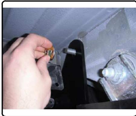
4. Torque all 9/16" fasteners to 150 lb-ft and all 1/2" fasteners to 110 lb-ft.
