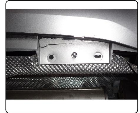
2. Remove (2) M10 bolts for the exhaust brackets. Lower the exhaust.
