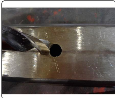
9. Fishwire (1) 1/2" carriage bolt and spacer from a hole approximately 6" forward of the forwardmost hole to the rearmost hole on each frame rail.
