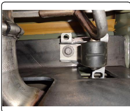
13. Torque all 1/2" bolts to 110 ft-lbs. Torque all M8 bolts to 48 ft-lbs.
