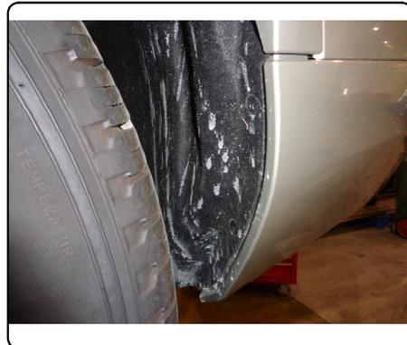
5. Gently remove bumper fascia, and detach sensors as needed. Mark sensors upon removal to ensure proper reattachment.
