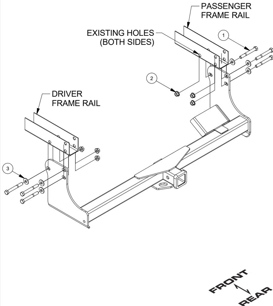
1. Locate tie-down loop on passenger frame rail and remove (2) M10 bolts on the bottom of the frame using a 16mm socket. Remove (2) M12 bolts on the inside of the frame using an 18mm socket and 18mm wrench. Return tie-down loop to owner.
