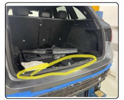
2B. Inside the rear cargo area, remove the floor pan to access the (2) electrical sensor plug. Locate electrical sensor plugs against the rear trunk wall, on the passenger side. Unplug the electrical sensor plugs. Dislodge the grommet and push to the rear/outside of the vehicle. These harnesses are connected to the vehicle fascia.
