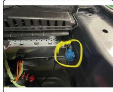
3. Remove lower rear fascia by locating and removing (6) screws (3) on each side using 10mm socket and (4) push pins (2) on each side using pry tool. Unclip electrical harnesses.
