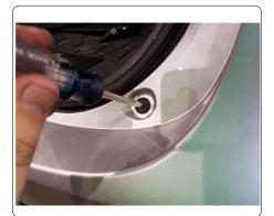
4. Gently remove the bumper fascia starting at the outside of the vehicle and working towards the rear of the vehicle. Locate on the bumper fascia and unplug (2) electrical plugs. Set aside for later reinstallation.
