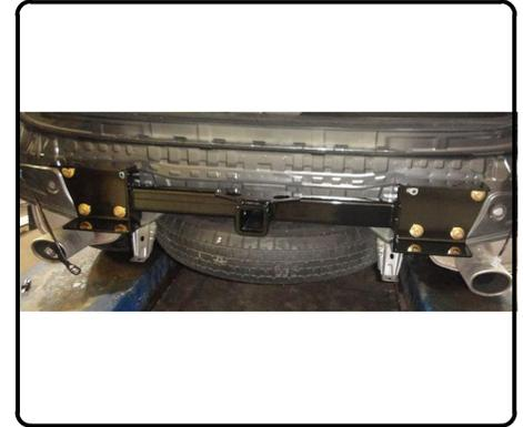
11. Reinstall fascia removed in STEPS 1-6 in reverse order. Be sure to reconnect the plugs that were disconnected during fascia removal process. **Note:** fascia has a removable panel for hitch usage. The panel can then be reinstalled when hitch is not in use.
