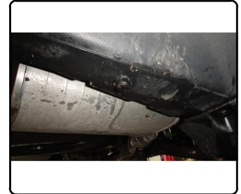
2. Remove splash guards by removing (2) bolts using an 8mm socket from each wheel well. Set aside for reinstallation in STEP 11.
