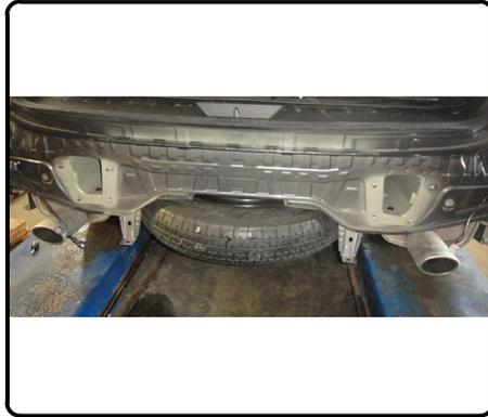
9. Using a hammer, bend bumper mounting flange inward toward the front of the vehicle to allow hitch to mount flush with vehicle.
