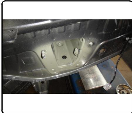
10. Raise hitch into position by placing over bumper studs. Secure the factory nuts that were removed in STEP 8. Install the supplied M10 bolts and conical washers. Attach wire harnesses to the top of the hitch and zip tie into place. Torque all M10 hardware to 48lb-ft
