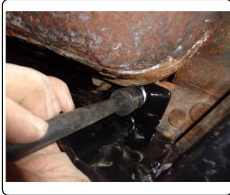
4. Raise gas tank pan by tightening the gas tank skid bolts with 18mm socket.
