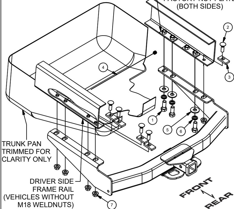
Note: Remove OEM Hitch prior to CURT hitch install.
