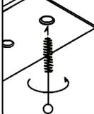
To remove debris from weldnuts in frame, spray lubricant or compressed air into hole. For heavy debris, use a small wire brush. (Be careful not to damage threads).
