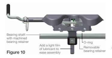
Ensure that the machined bearing retainer and the removable bearing retainer are against lower bearing assembly. Both sit inboard of mid-section bearing shaft cradles during assembly.
