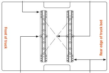
Each base rail must have a bolt in either of the marked holes. Check for obstructions before drilling
