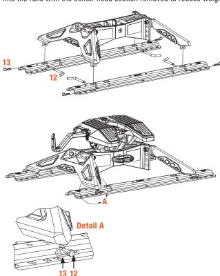
If installing new base rails, follow the instructions provided by the rail manufacturer for proper placement, alignment and spacing per your vehicle's year, make and model. If the 5th wheel is being mounted to existing base rails, and alignment issues arise, it may be necessary to proceed as follows:
