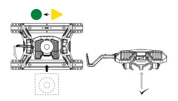
If the kingpin is resting on top of the jaws, immediately lower the trailer jacks to lift the kingpin off the jaws. Inspect the 5th wheel for damage that may have resulted from the improper coupling attempt. Under no circumstances should the 5th wheel unit be used if damage exists. If no damage exists, review coupling instructions and repeat procedure.
