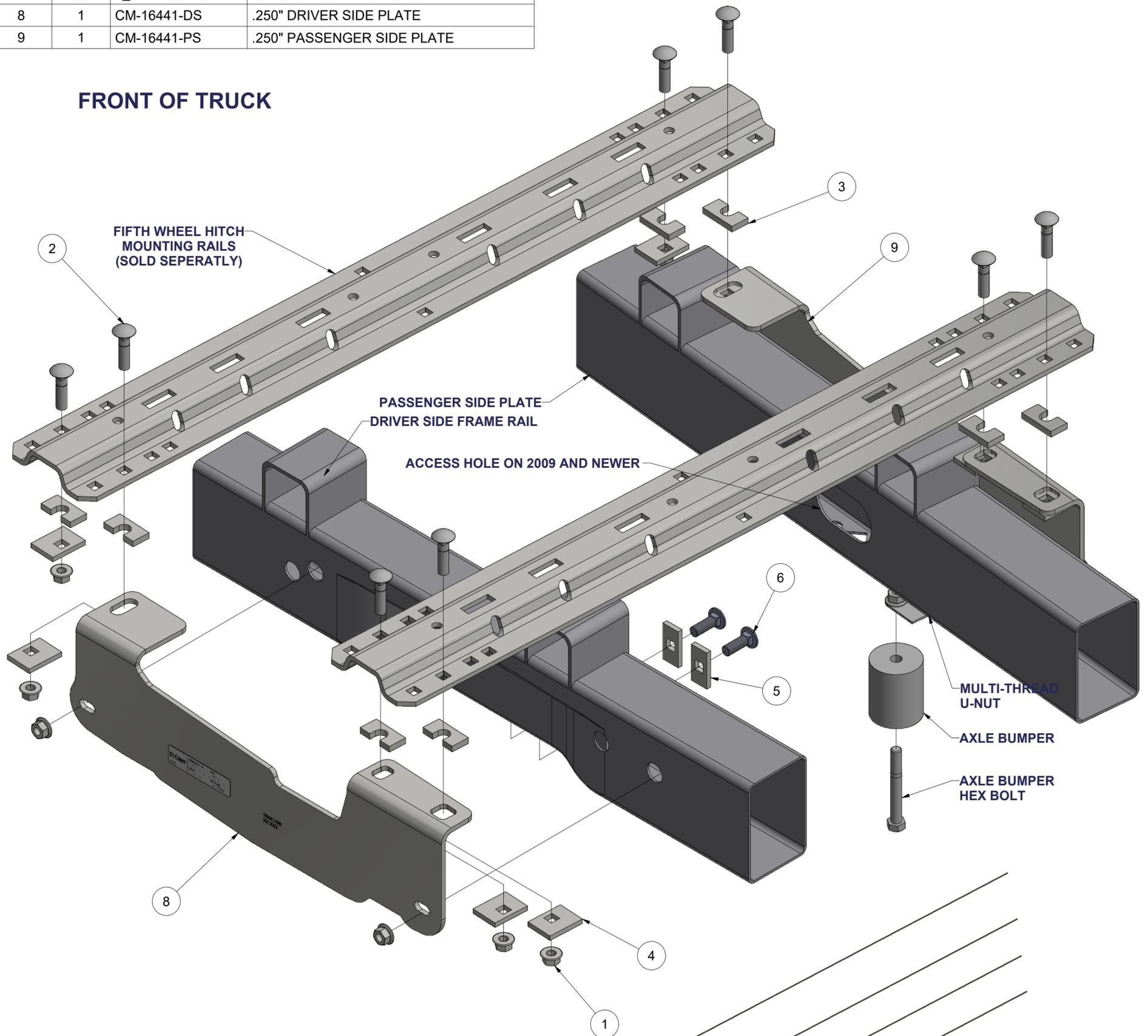
REMOVE THE AXLE BUMPER, MULTI-THREAD U-NUT,
