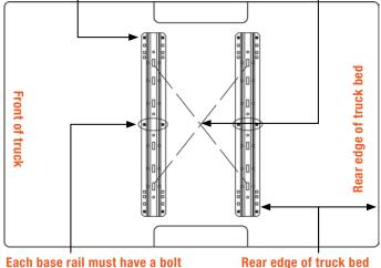
Each base rail must have a bolt in either of the marked holes. Check for obstructions before drilling
