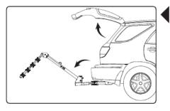
At the base, remove the clip from the upper bolt holding the bike rack in the vertical position. Remove the bolt and tilt the rack away from the vehicle. The rear cargo area is now accessible.
