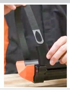
Orientate the tray assembly with the CURT logo onto the shank assembly (#2) as shown. Align the tray holes with those in the shank assembly. Place a tray spacer (#5) onto the tray, aligning its holes with those in the tray. Insert two 3/8" carriage bolts (#12) through the spacer, tray and shank assembly. Place a 3/8" flat washer (#13) and 3/8" nylock nut (#14) onto each bolt.
