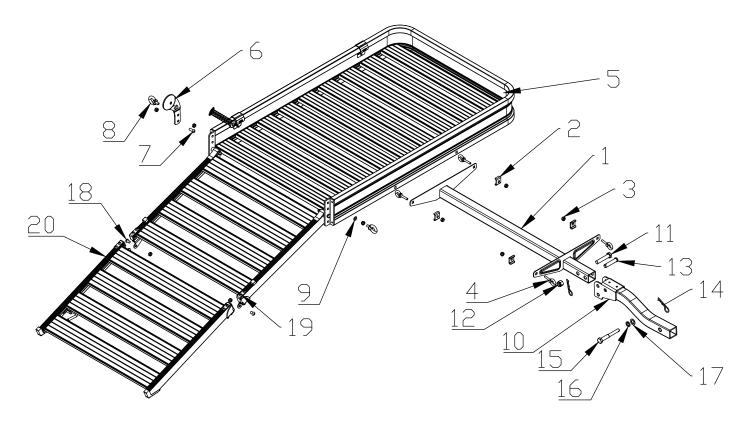
Align the holes in the upper ramp (#19) and lower ramp (#20) hinge brackets. Insert an M10 button socket cap screw (#18) into each hinge. Secure with an M10 lock nut (#3), ensuring the hinge operates freely.
