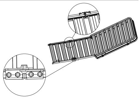
Place the bottom bracket (#1) on the bottom of the carrier frame (#5) and line up the square holes.
