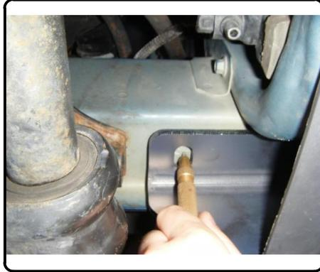
4. Drill holes marked in Step (3). Enlarge the drill hole in the passenger side frame rail to allow 7/16" carriage bolts and SP11 spacers to pass through. **Note:** If existing access hole is not present in driver side frame rail, enlarge the drill hole to allow 7/16" carriage bolts and SP11 spacers to pass through.
