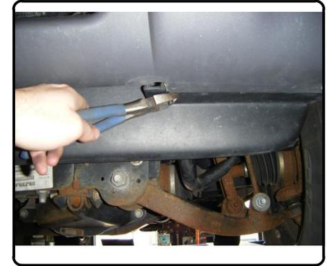
2. Mark and trim the plastic wheel well. **Note:** Dimensions are approximate, confirm fit before trimming.
