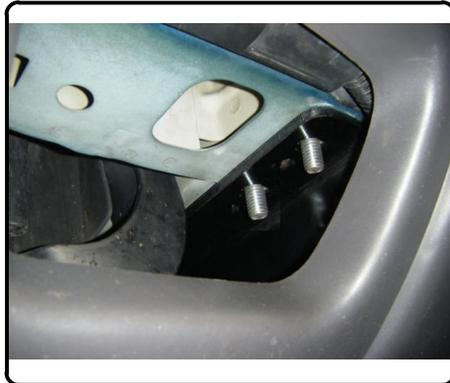
8. Reinstall the (2) screws removed in Step (1) and secure the bumper cover to the radiator support bracket.
