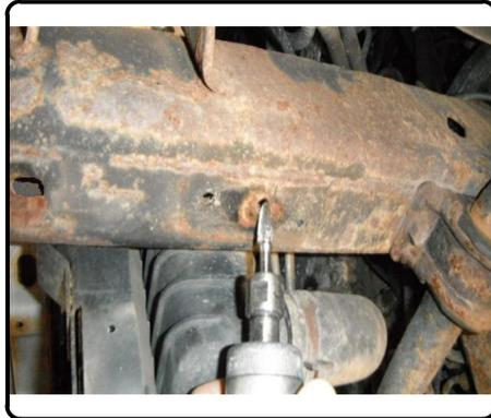
4. If access holes are not present, enlarge the forward most mounting hole on each frame rail so that 1/2" hardware will pass through.
