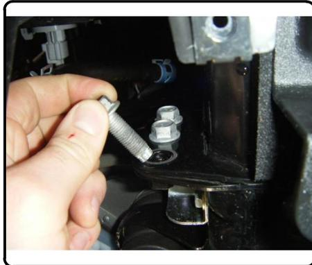
3. Lift hitch into position, locating the vehicle tow loops under the hitch mounting plates.
