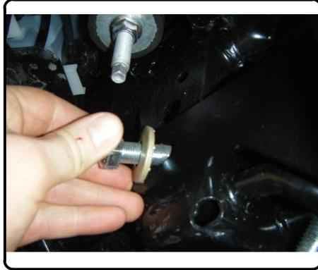
6. Insert 5/8" carriage bolts through the hitch mounting plates and tow loops. Secure hitch to tow loops by attaching supplied spacers and 5/8" flange nuts to carriage bolts.
