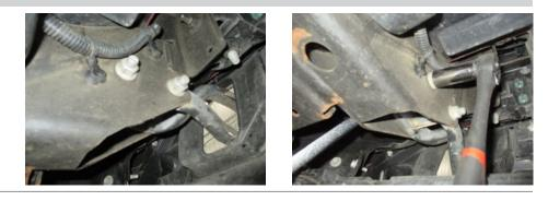
Use a small pry tool to remove the rearmost wire harness clip on the inside of the frame on the driver side.
