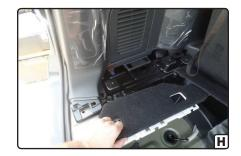
Remove the center trim piece of the rear scuff panel (C). Remove the scuff panel by pulling out on the bottom and then up. Take care not to damage the alignment tabs on the back (D).
