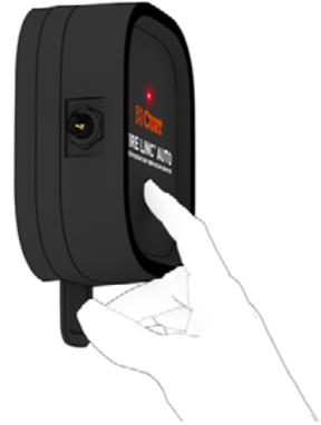
The LED will begin to flash 10 times as it completes the factory reset. When factory reset is complete, the LED will turn off.
