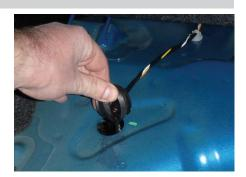
Using a rotary tool, cut a relief in the trunk pan hole just big enough to get the 4-flat through the grommet hole.
