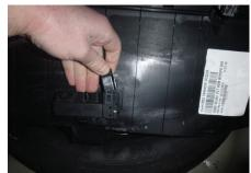
Starting on the passenger side, remove the cargo net hooks. These hooks will have threads securing them into place on the side panels.
