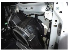
Locate the gray housing similar to that of the custom RV harness. Separate the connectors, taking care not to damage the locking tabs. Insert the custom RV harness end with the green wire between the separated connectors. Make sure the connectors are fully inserted with locking tabs in place.
