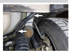
From the front of the tank, route the 4-flat wire around and in-between the fuel emissions canisters. Proceed to follow the brake lines to just behind the front tire.
