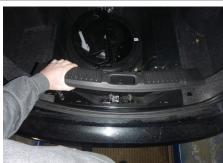
Use a panel trim removal tool to remove the push fasteners from both sides of the trunk.
