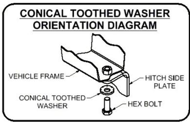
**PERIODICALLY CHECK THIS GOOSENECK HITCH TO ENSURE THAT ALL FASTENERS ARE TIGHT AND THAT ALL STRUCTURAL COMPONENTS ARE SOUND.**
