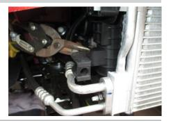
Use a 3/8" drill bit to drill the forward-most top holes. Fishwire the 3/8" carriage bolt (#6) and square hole spacer (#10) into the frame and through the baseplate and secure with 3/8" serrated-flange nuts (#8).
