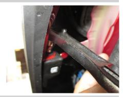
Use a T-15 Torx to remove the eight bolts from the bottom of the bumper cover, two on each side and four in the center.
