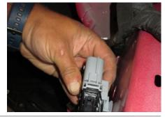
Unclip the wire harness on the driver side of the vehicle and trim the shutter mounting flanges as needed on both sides.
