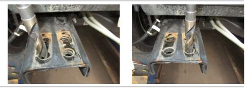
Slide the baseplate (#1, #2) on top of the frame and align with the existing front tow hook holes. Install two of the  $5/8" \times 1-3/4"$  hex head cap screws (#6) and washers into the holes previously enlarged. Secure with 5/8" serrated flange nuts (#8).
