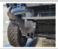
With the 10mm bolts snug on the front of the baseplate, fully tighten the M12 bolts on the side of the baseplate on both sides of the vehicle to 55 ft-lbs.
