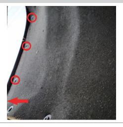
Gently pull outward on the fender flare to access and remove the T-15 screws.
