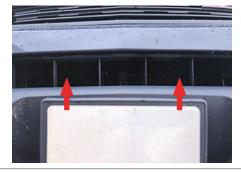
Using a 15mm socket, remove the outer-most bolt from both sides of vehicle.
