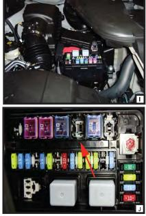
7. On the driver's side under the hood, locate the fuse box and remove black plastic cover (I). Insert 20 amp SLO-BLO fuse into position as shown (J).
