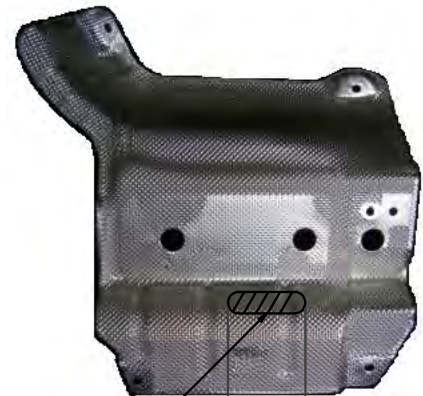
MUFFLER HEAT SHIELD TRIMMING DIAGRAM
