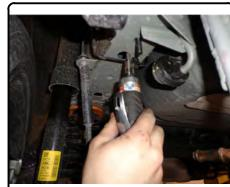
4) Fishwire spacers and 7/16" bolts through access holes and into the bottom mounting holes in the vehicle frame. Raise hitch into position and loosely secure in place with the 7/16" nuts provided.
