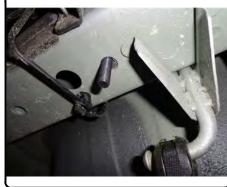
5a) If no weldnuts exist in frame, fishwire the hardware for the vertical mounting points through the framerail and the hitch side plates. Secure all 7/16" hardware.b) If weldnuts exist in frame, then secure hitch with M12 bolts and 1/2" conical washers in the side mounting plates
