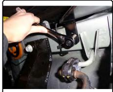
6) Torque all 7/16" hardware to 70 lb-ft. Torque all M12 hardware to 86 lb-ft. Raise exhaust hangers back into position.
