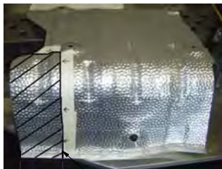
HEAT SHIELD TRIMMING DIAGRAM
