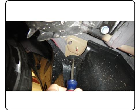
2. Using a 12mm socket, remove the (8) bolts attaching the bumper assembly to the rear face of the cabin. Lightly pull the lower fascia away to remove the bumper beam and return flange bolts to vehicle owner.
