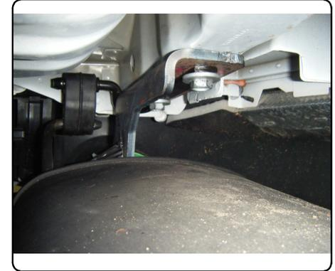
6. Re-attach (2) center rubber exhaust hangers which were removed in STEP 1.
