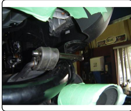
4. Use included hardware to attach hitch and exhaust hangers to vehicle frame. Leave bolts loose. **Note:** Hitch is sandwiched between frame and exhaust hanger.
