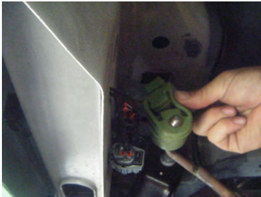
EXHAUST HANGER REMOVAL
