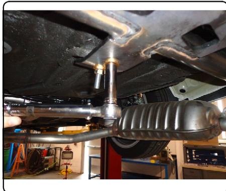
5. Raise exhaust back into position by connecting the rubber isolators on the muffler to the hanger studs on the hitch, and reconnect the center isolator. Reconnect exhaust tips removed in step (1)
