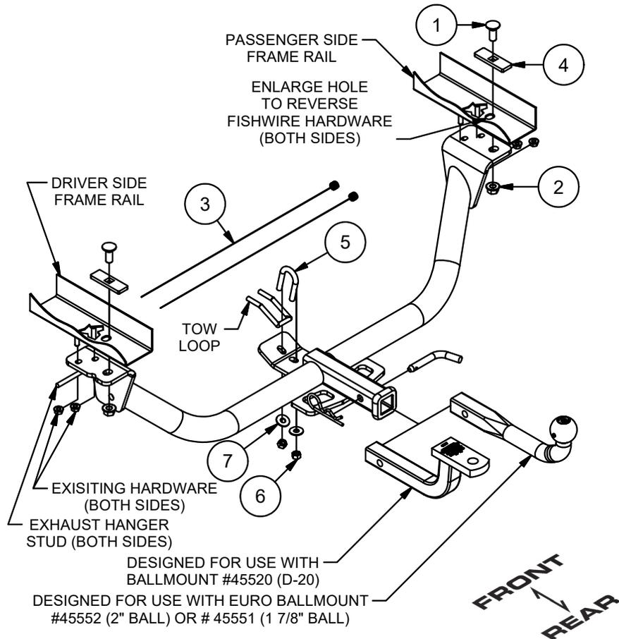
1. Lower exhaust by removing (4) screws with a 10mm socket connecting the exhaust tip to the fascia and push aside. Disconnect (2) rubber isolators located rear of muffler and (1) at the center of the vehicle.
