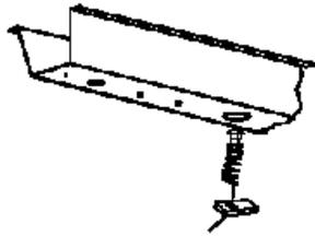
4. Raise hitch into position by loosely securing with the 1/2" hardware, and loosely secure tow loop attachment with 3/8" u-bolt, conical washers, and 3/8" nuts. Torque M8 hardware to 25 ft-lb, 3/8" hardware to 30 ft-lb, and 1/2" hardware to 110 ft-lb.
