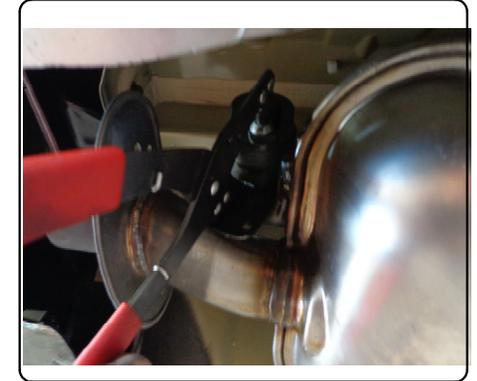
2. Unbolt exhaust hanger brackets (both sides), by removing (2) M8 nuts from each bracket. (Return bracket to customer)
