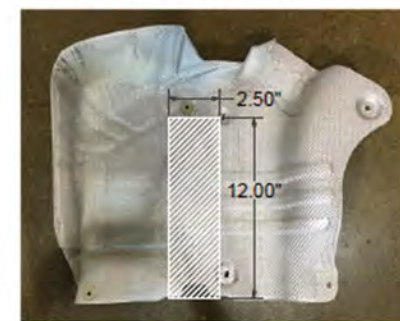
HEAT SHIELD TRIM DIAGRAM
