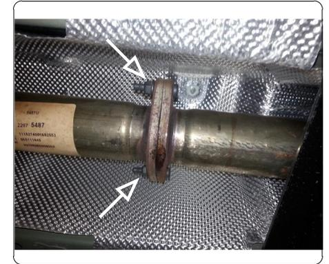
**2. On Malibu models only:** Separate exhaust flange and carefully slide the exhaust forward out of the rear bumper exhaust hangers. Set aside exhaust for later reinstallation. Remove the inside lower bumper bolts on each side of the vehicle using a 15mm socket. Replace with the supplied M10 bolts.
