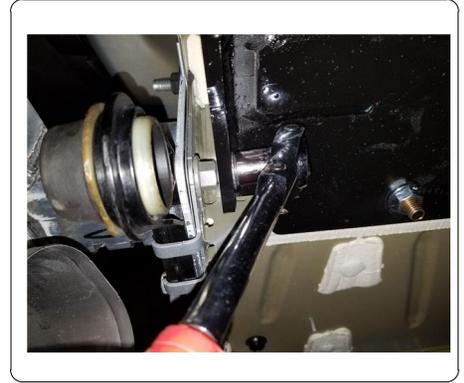
6. Torque all 7/16" hardware to 60 ft-lbs. Torque all M10 hardware to 45 ft-lbs. Reinstall exhaust and hardware removed in steps (1) and (2) in reverse order.
