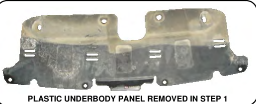
PLASTIC UNDERBODY PANEL REMOVED IN STEP 1
