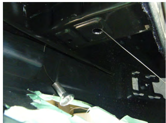
DRIVER SIDE FISHWIRE LOCATION
